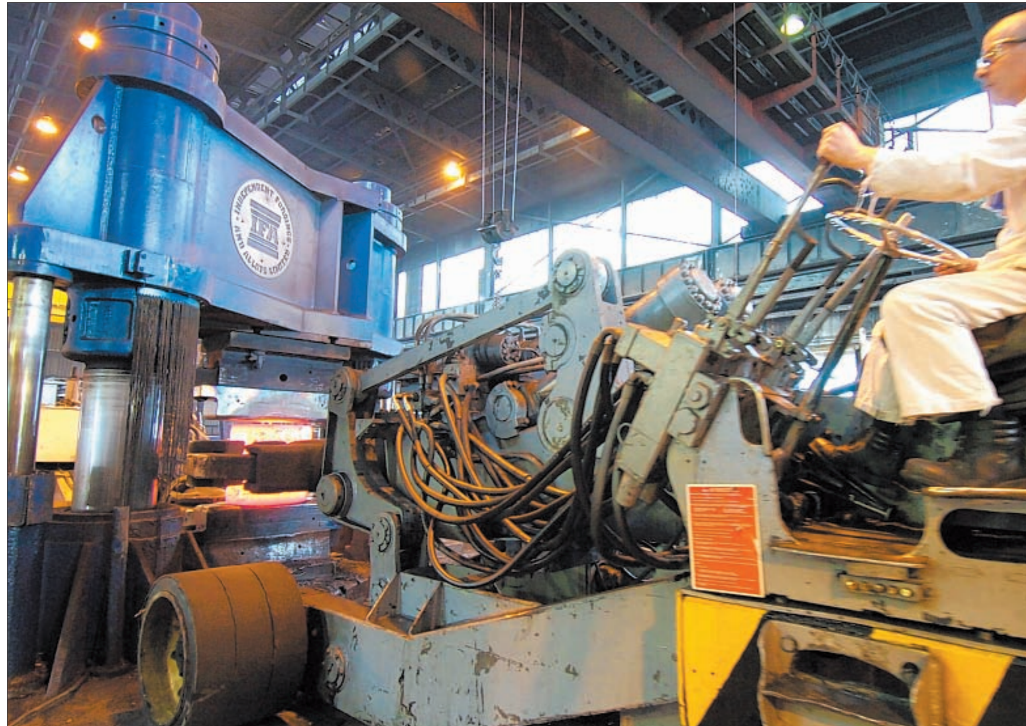
▲ Moving the metal: Driver Mark Woodhouse manoeuvres a huge hot piece of metal with towards the 1500-tonne open-die press with a giant machine
