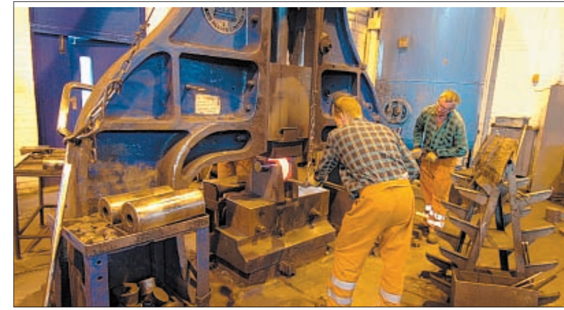
▲ Skilled manpower: Two men operating the ring drop-hammer forge at IFA
